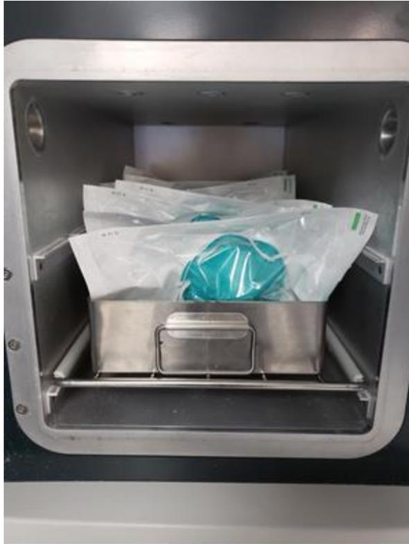
**Figure 4:** Sterilization basket with up to 12 individually packaged respirators, placed inside of the Sterilucent sterilizer.
